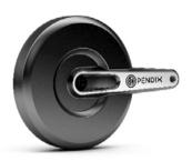
The Pendix motor is an efficient, high-power direct drive system, working without gears or freewheeling. Its control is already integrated in its smart design. The Pendix motor is located on the left side of the bicycle directly on the supplied electronic bottom bracket, which identifies the force exerted through pedaling. The motor then supports you corresponding to the settino/mode you have selected.
